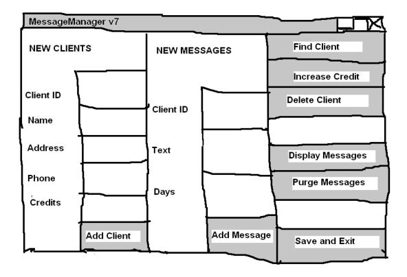
This is made up of three areas. From left to right these are a) an area for adding new clients, b) and area for adding new messages and c) an area for buttons dedicated to other essential operations.
